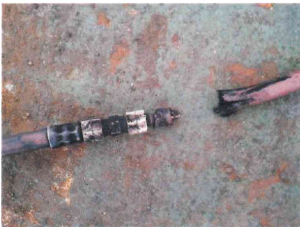
Damaged hoses after fire
